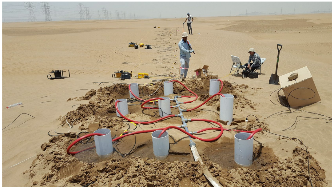
Figure 2. Photograph of the field experiment where the seismic data are recorded over the sand dune during the injection of 12-tons of water.
