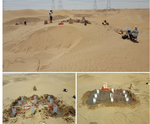
Figure 2: Photos of the field site, where 12-tons of water were injected into the subsurface.
