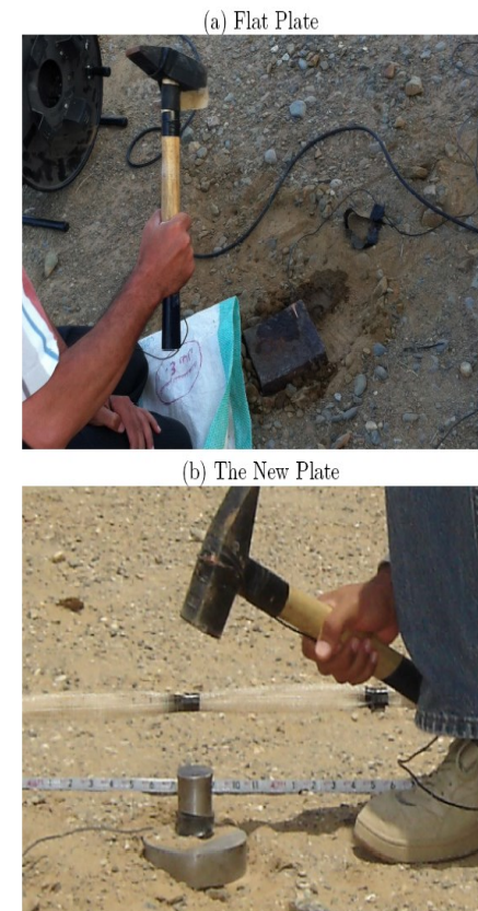
The plates used with seismic source: (a) The flat plate, and (b) The plate used to maximize source repeatability and minimize bouncing
