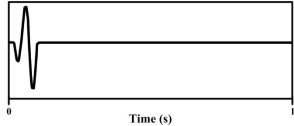
Figure 4: Source wavelet used in EWI. We extracted it from the recorded data by averaging 10 to 20 near offset first arrivals aligned by cross-correlation
