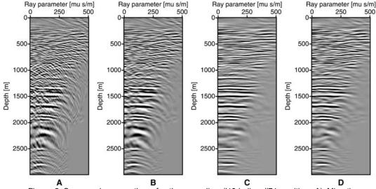
Figure 2 Common image gathers for the cross-line #10-in-line #71 position. A) Migration result. B) Regularized LSM after 4 CG iterations. C) Regularized LSM after 11 CG iterations D) Preconditioned LSM after 4 CG iterations.
