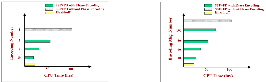
Figure 6.9: (Top). CPU time comparison for encoded SSF+FD migration with different number of shot gathers; Encoding Number denotes the number of adjacent shot gathers to be phase encoded. (Bottom) CPU time comparison for encoding SSF+FD migration with the second strategy. Note, the CPU time of no-encoding SSF+FD migration and Kirchhoff migration are also presented for comparison.
