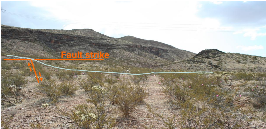
Figure 2.2: View of the Washington fault scarp and 2-D seismic survey line. The yellow line represents the fault strike direction, and the green line represents the 2-D seismic survey line.
